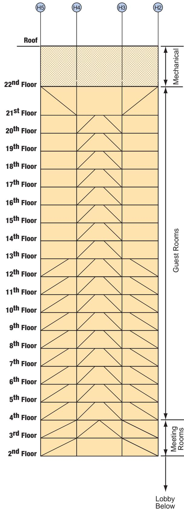
Figure 3-5 Typical transverse bracing elevation (Weiskopf & Pickworth 1979b).
