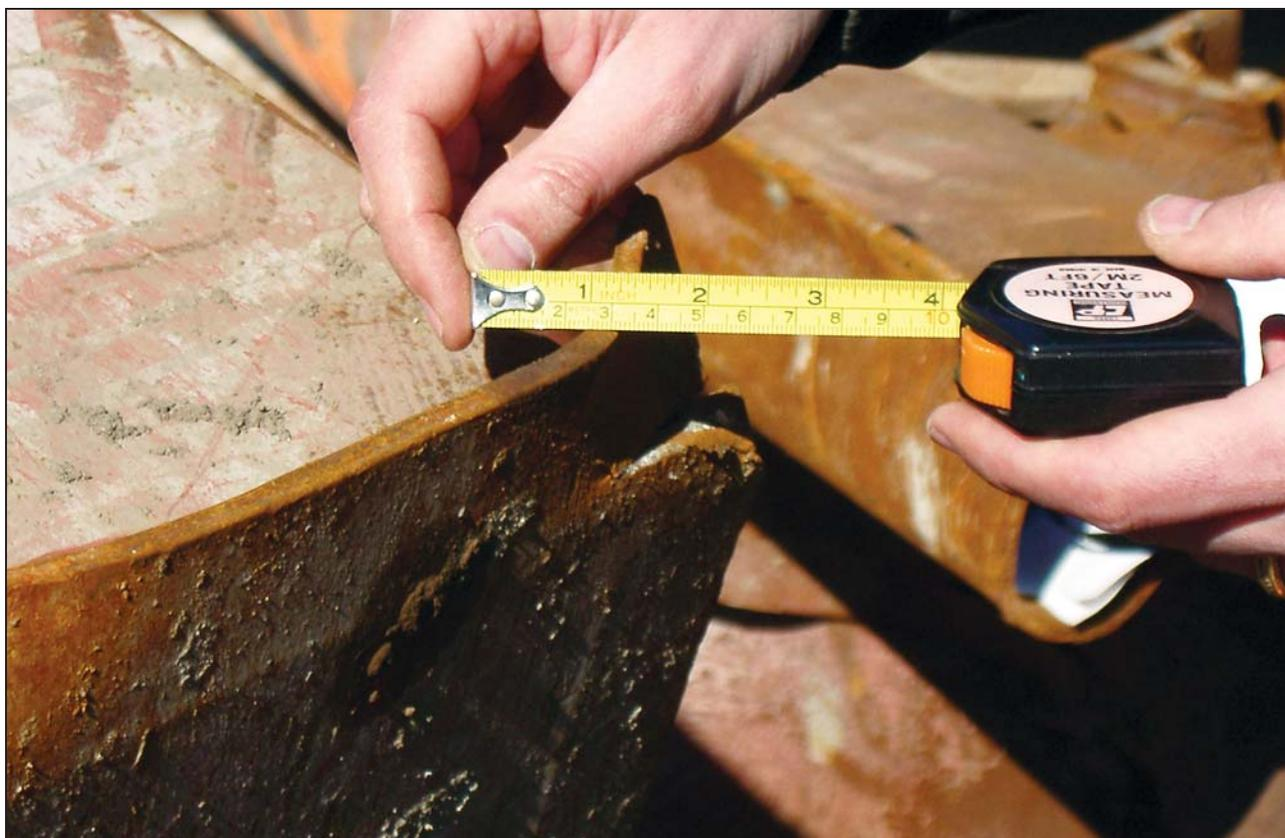
Figure D-9 Measurement of 1/4 inch for web thickness ( $t_w$ ).
