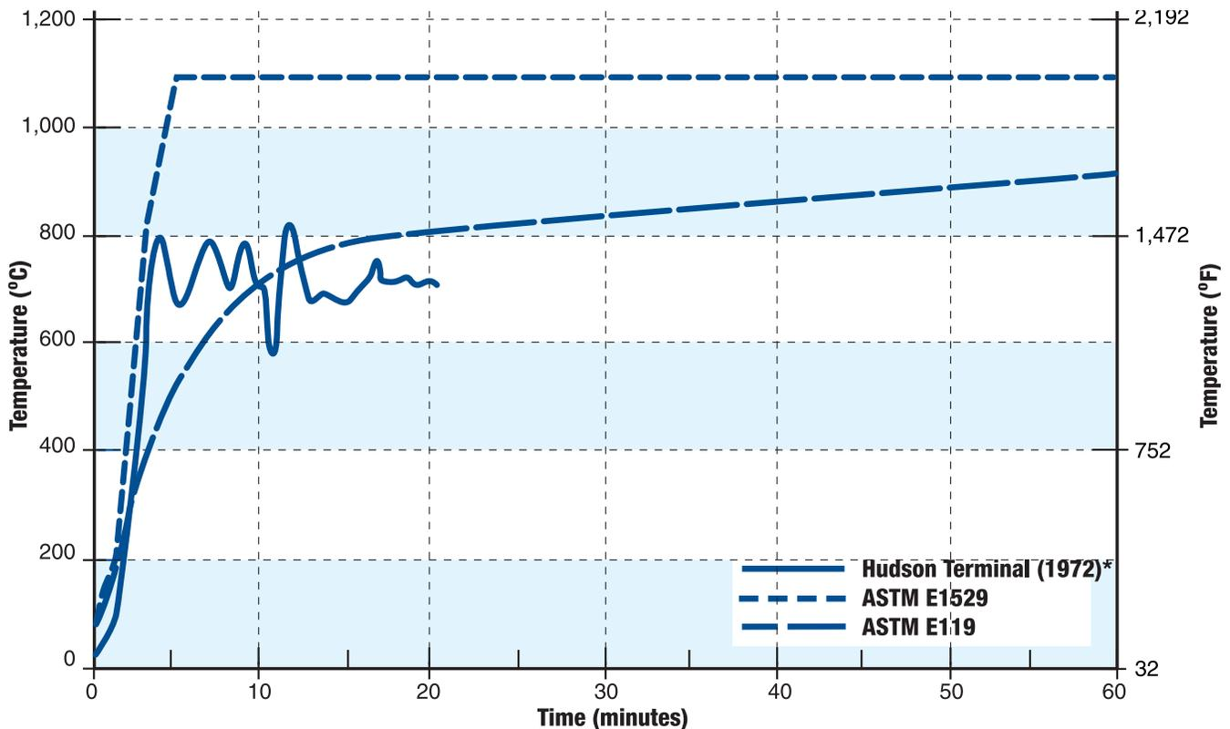
\*Hudson Terminal experiment conducted with normal office fuel load (6 psf) (DeCicco, et al. 1972)
