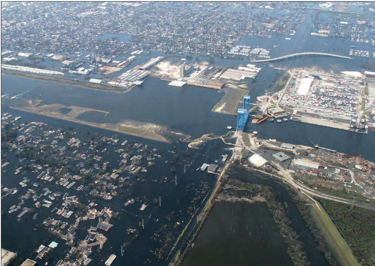
Figure 8-5. The Industrial Canal levee breach in New Orleans
