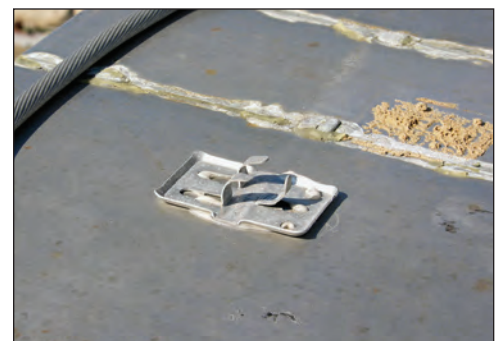
Figure 3. During high winds, the conductor deformed the prongs and pulled away from this conductor connector.
