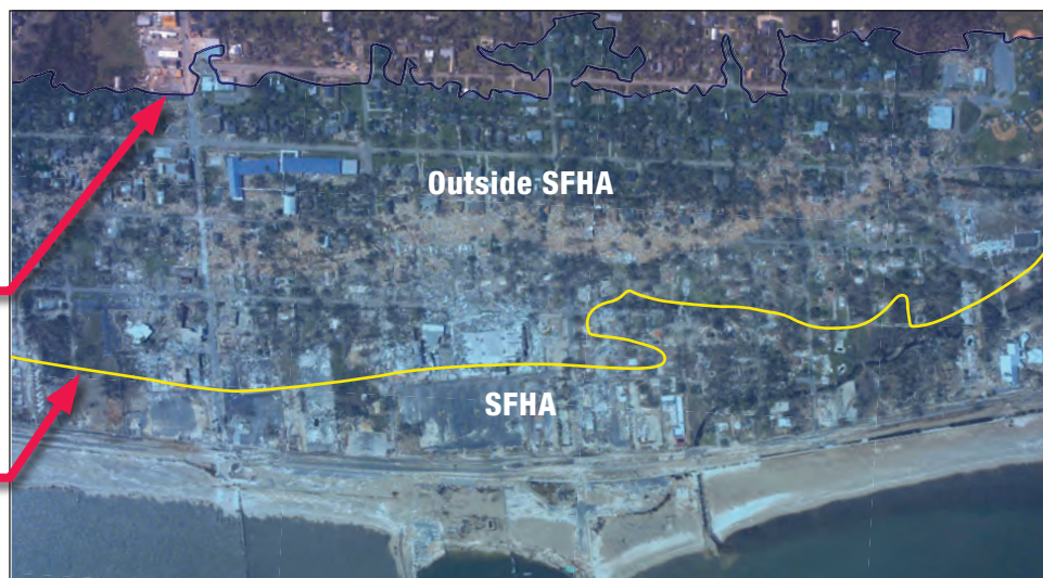
Figure 2. Map showing storm surge inundation by Hurricane Katrina at Long Beach (blue shading). Katrina flooding extended beyond the limits of the mapped 100-year floodplain (SFHA) (photo source: NOAA).
