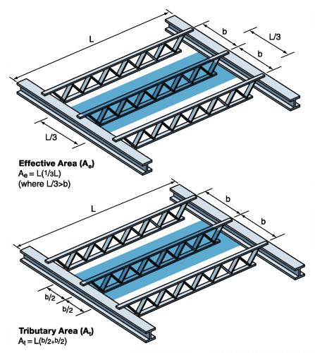
Figure B3-4: Comparison of tributary and effective wind areas for a roof supported by open-web steel joists
