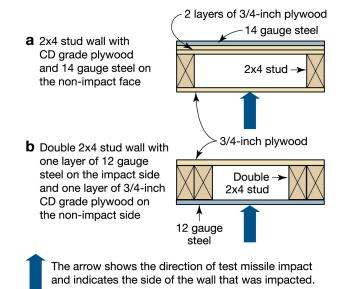
Figure B8-12: Use of steel sheet metal in wall assemblies
