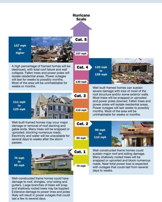
Figure A2-4: Typical hurricane damage descriptions to one-and two-family dwellings and thier corresponding intensity accordig to the Saffir Simpson Hurricane Wind Scale
