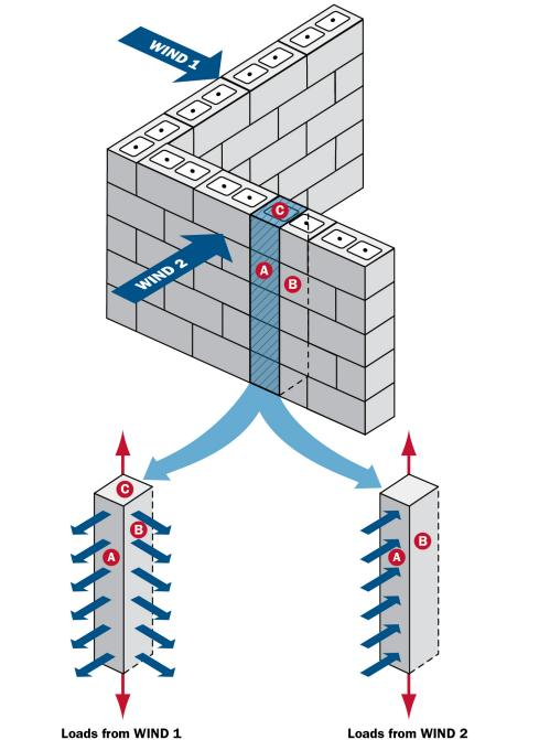
Figure B3-5: MWFRS combined loads and C&C loads acting on a safe room wall section
