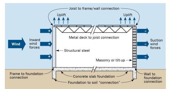
Figure B3-6: Critical connections important for providing a continuous load path in a typical masonry, concrete, or metal-frame building wall (for clarity, concrete roof deck is not shown)
