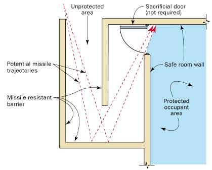
Figure BB3-18: Alcove entry system protected by a debris-resistant barrier (note that the safe room roof extends past the safe room wall and connects to the top of the debris-resistant barrier to prevent intrusion of debris traveling vertically)
