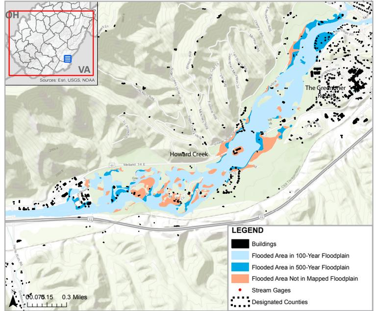
FIGURE 6: Inundated area along Howard Creek, between White Sulphur Springs and Caldwell, West Virginia.
