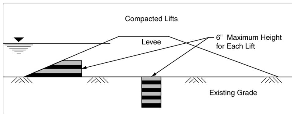
**Figure 5-2. Levee construction**
