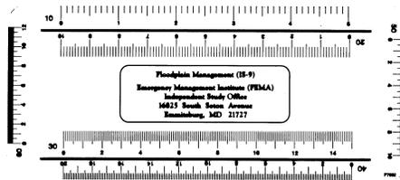
The clear plastic engineer's scale is included for use in some of the exercises in this course. It helps relate distances on the ground to measurement on a map.
