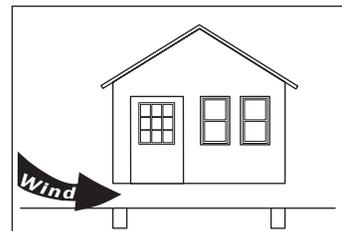
Uplift failure mode is particularly likely when the 3-foot pier rule is used in areas where the BFE is greater than 3 feet above the ground elevation. In that situation, the home will become submerged and exposed to buoyancy forces. For relatively low levels of flooding (9 to 12 inches or less), buoyancy forces can exceed the weight of the home and lift the home off its foundation. To resist buoyancy, foundations must provide sufficient resistance to overcome buoyancy (and
