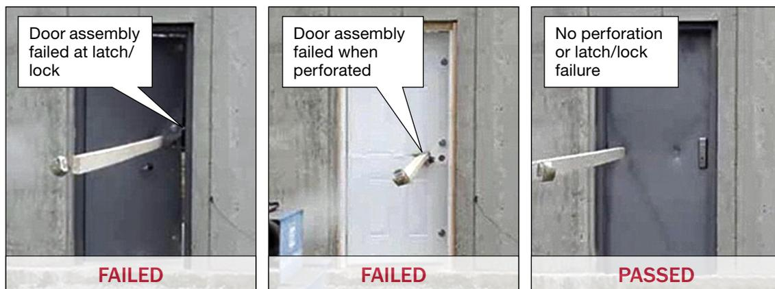
Figure 2: Examples of doors that failed or passed testing
