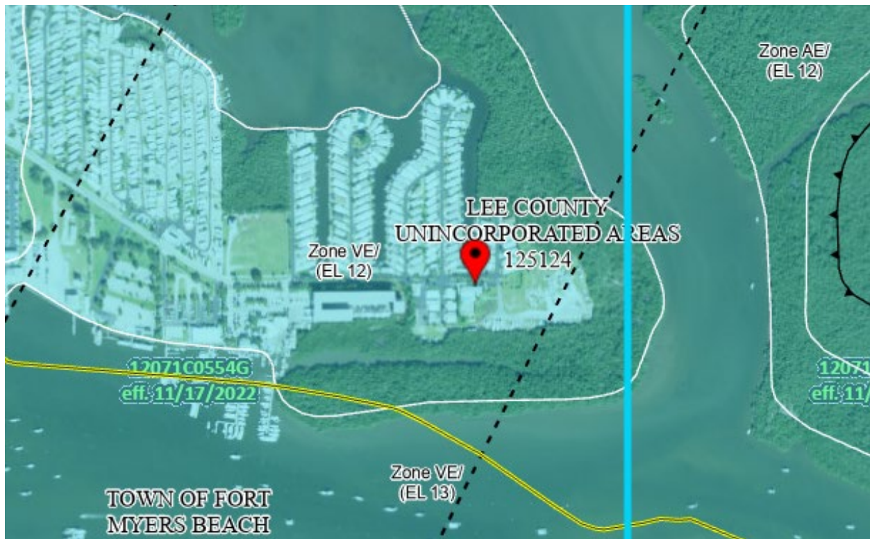
Figure 3-124: New 2022 FIRM for Port Carlos Cove that went into effect after Hurricane Ian (Lee County, Zone VE)
