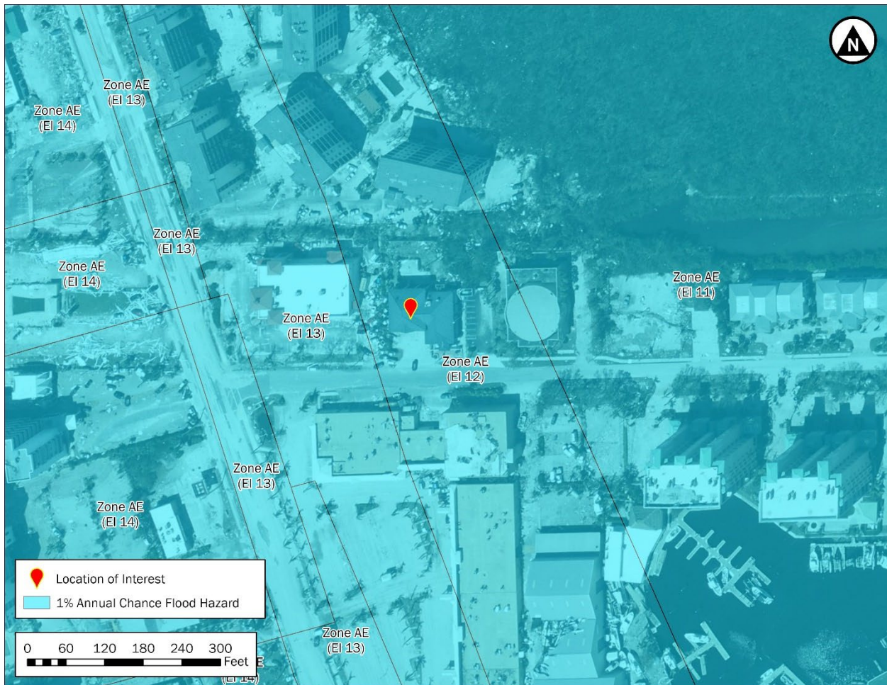
Figure 5-28: Effective FIRM at the Fort Myers Beach Fire Station #33 location at the time of Hurricane Ian’s landfall
