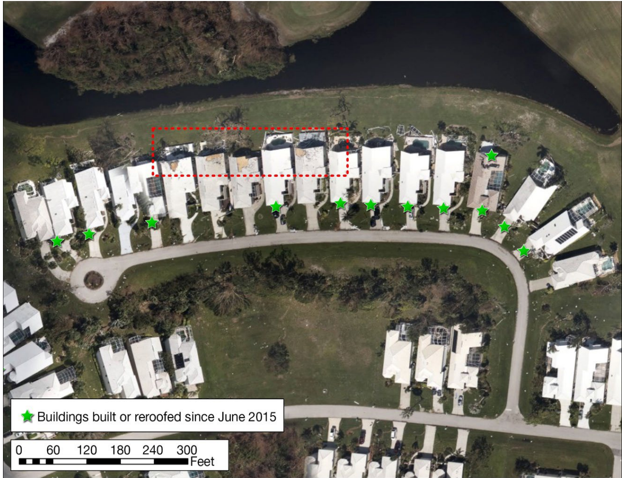
Figure 4-39: Roof tile damage on newer and older roofs (EWS = 126 mph) (Placida)
