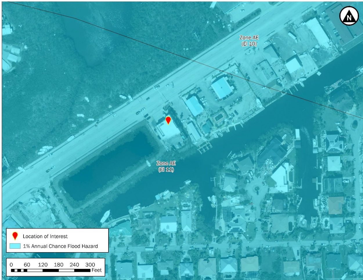
Figure 5-32: Effective FIRM at the Fort Myers Beach Fire Station #32 location at the time of Hurricane Ian’s landfall
