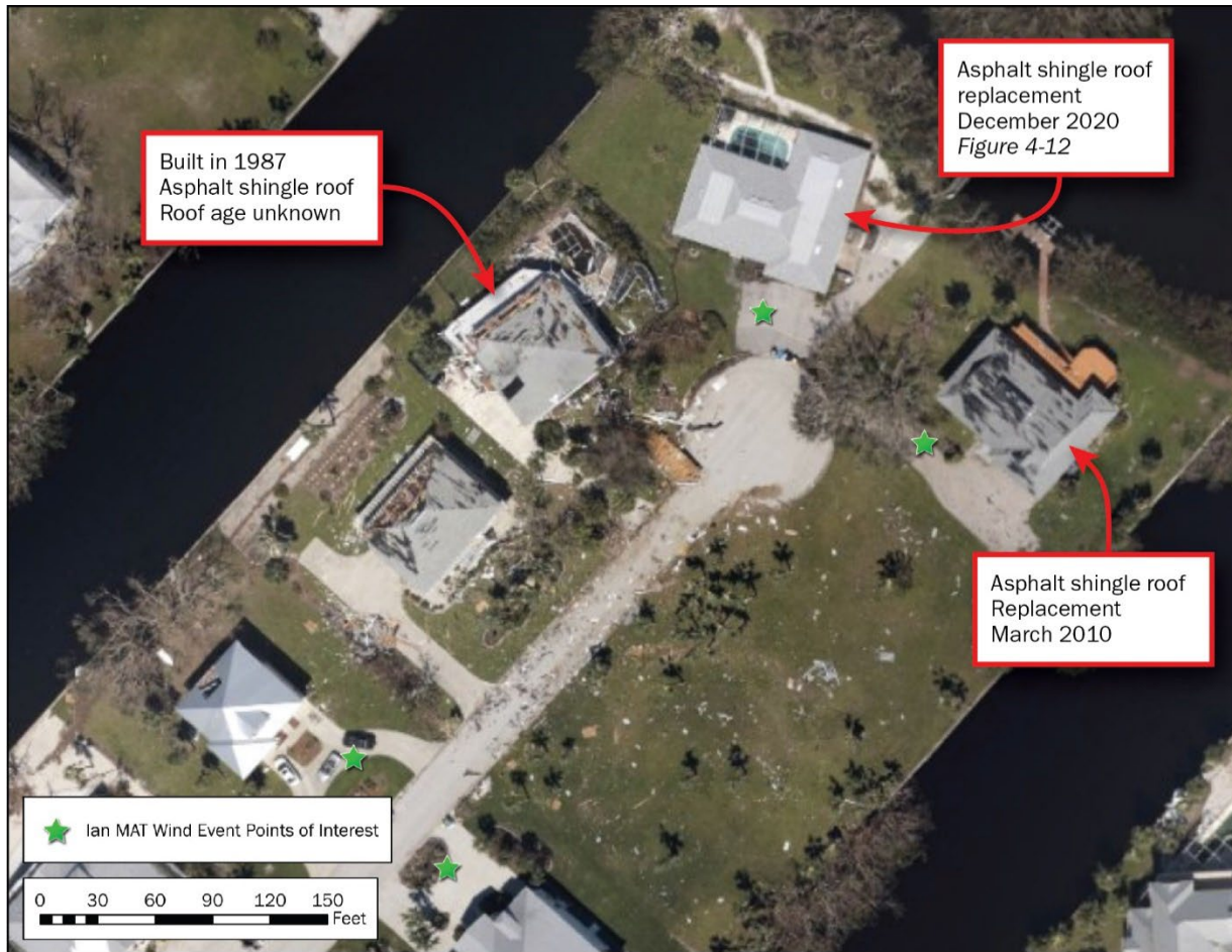
Figure 4-13: NOAA imagery of asphalt shingle damage on houses adjacent to the house shown in Figure 4-12 (EWS = 128 mph) (Placida)
