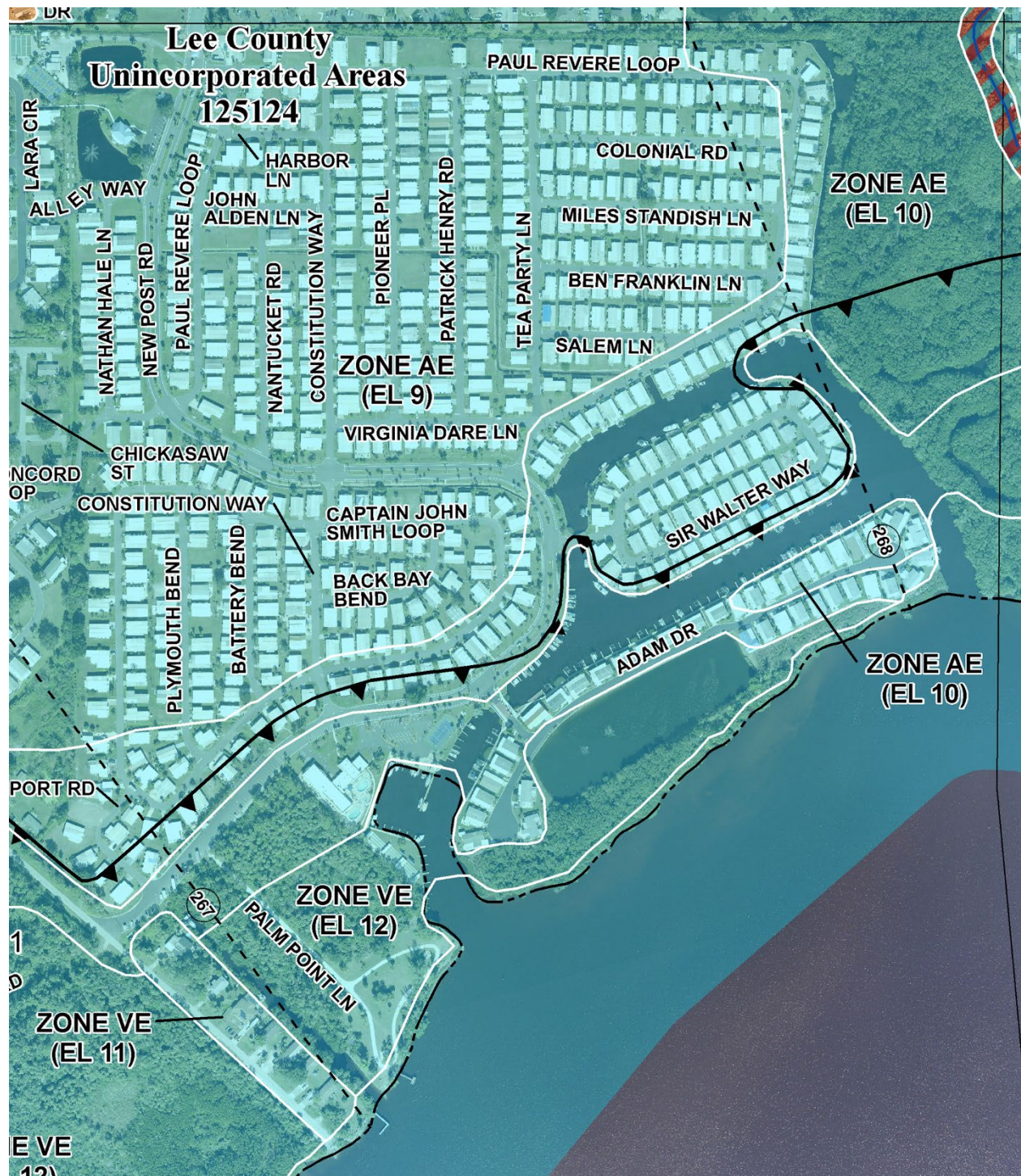
Figure 3-113: The November 2022 effective FIRM for the Old Bridge Village includes a LIMWA (Lee County, Zone AE & VE)
