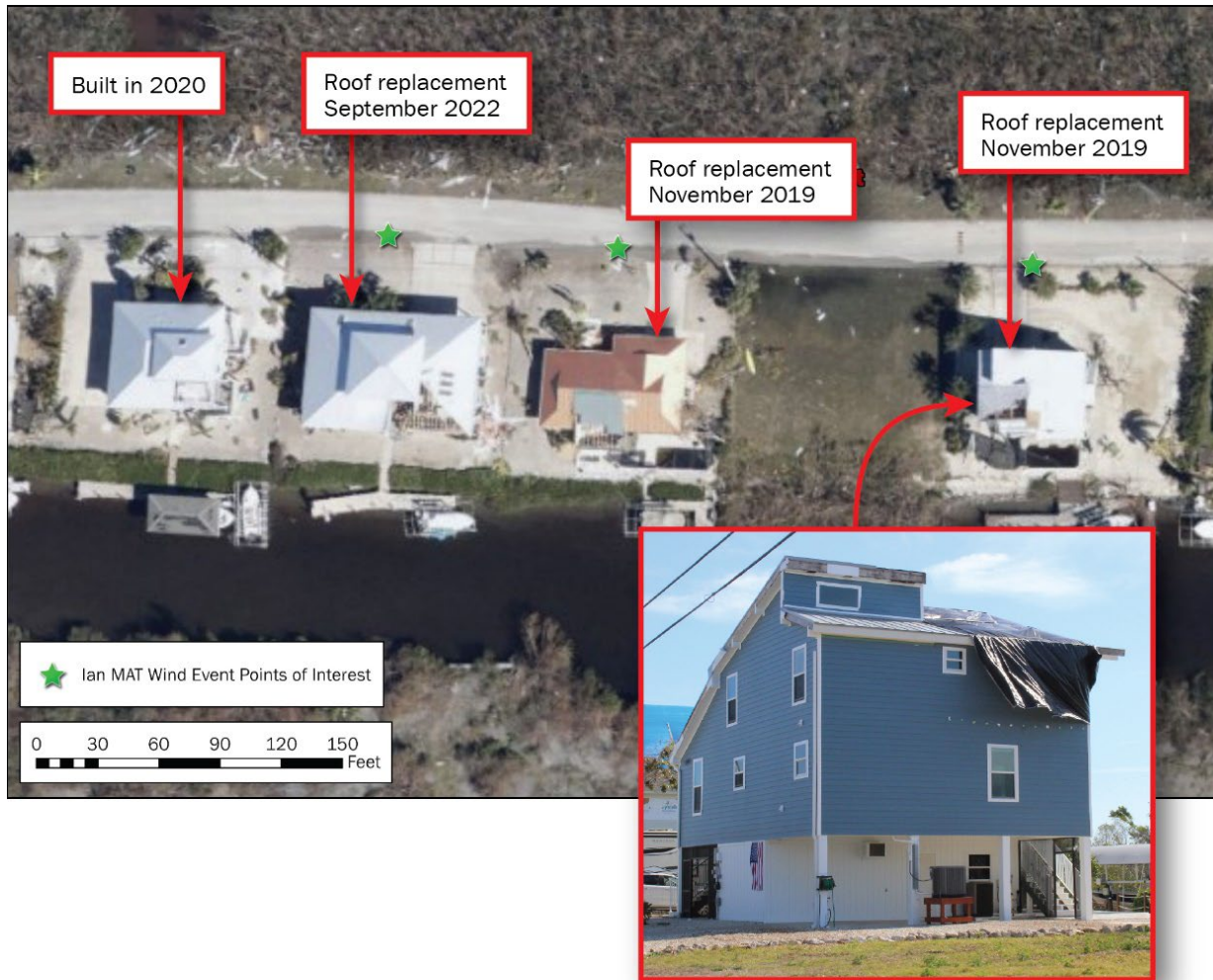
Figure 4-28: Metal panel roof cover damage on roofs that were recently replaced (EWS: 115 mph; DWS: 160 mph) (St. James City)
