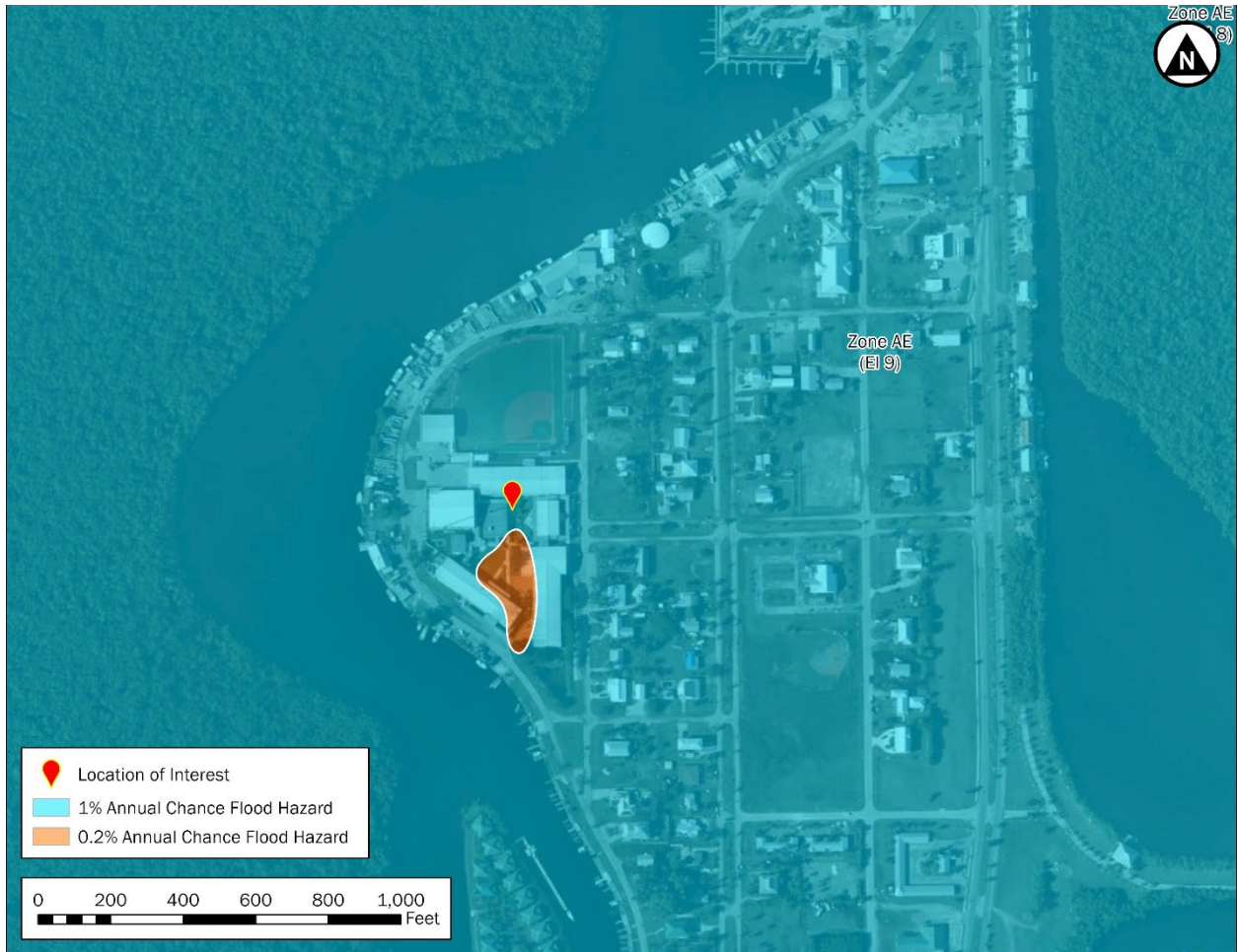
Figure 5-75: Effective 2012 FIRM at the Everglades City School location at the time of Hurricane Ian's landfall
