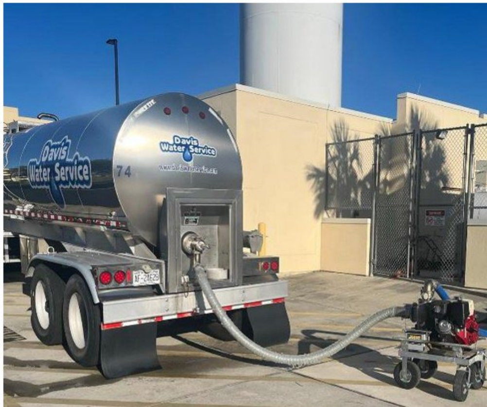
Figure 5-4: Potable water truck and pump supplemented on-site stormwater for operating HVAC equipment and flushing toilets (Lee County)
