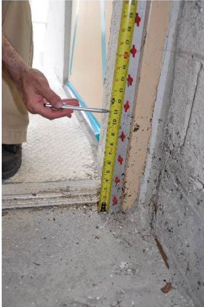
Figure 3-88: HWM observed at the Fort Myers Beach Library lowest floor of the 1994 building (Lee County, Zone AE)
