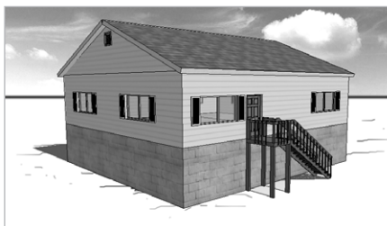
Two floor building with a full floor solid perimeter foundation for the first story and a frame construction for the second floor.
