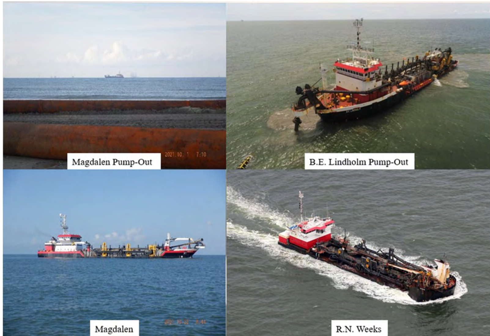
Figure 2. Typical Hopper Dredges.
