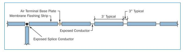
Figure 3-98: Plan showing conductor attachment
