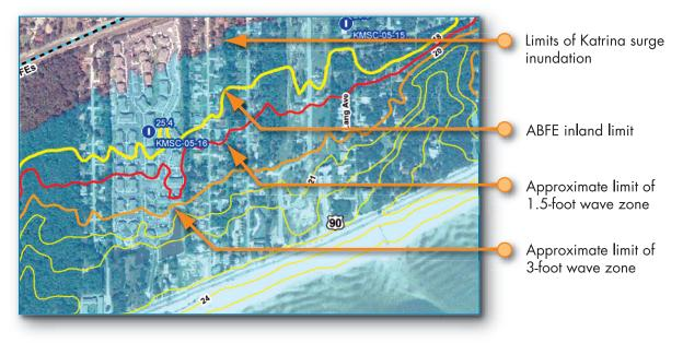
Figure 2-5: Example of a flood recovery map showing ABFEs and other flood hazard information.
