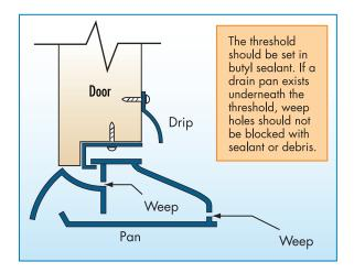
Figure 3-35: Interlocking threshold with drain pan
