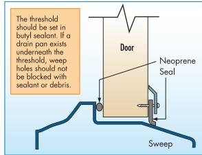
Figure 3-36: Threshold with stop and seal
