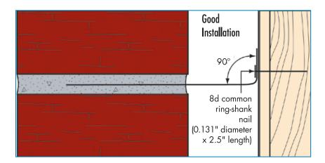
Figure 3-50: Bend ties at nail heads
