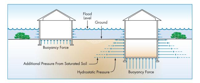
Figure 2-8: Hydrostatic loads on buildings
