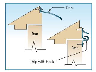
Figure 3-32: Drip at door head and drip with hook at head
