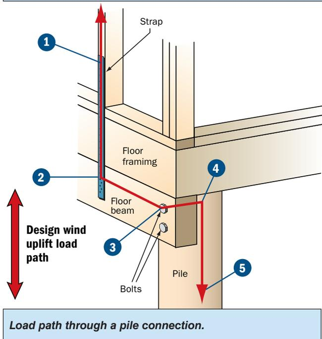
Load paths can be complex through a connection. It is important that each link within the connection be strong enough to transfer the full design load.
