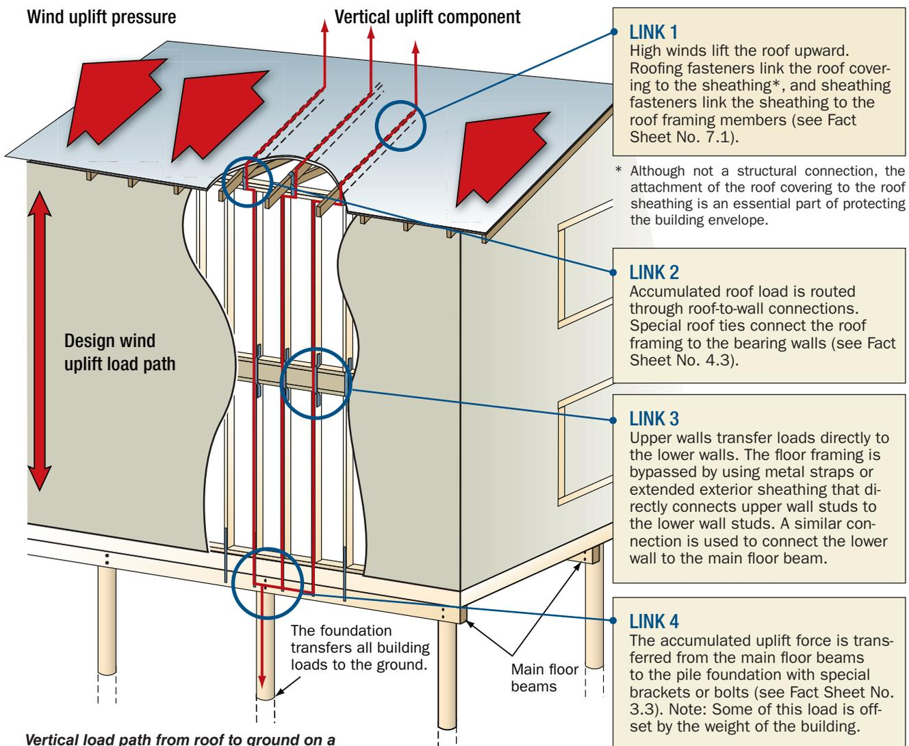
**Vertical load path from roof to ground on a platform-and-pile-construction building. Note: Load paths will vary depending on construction type and design. Adjacent framing members will receive more load if a connection fails.**
