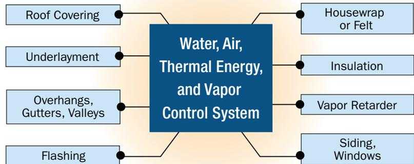
The purpose of the building envelope is to control the movement of water, air, thermal energy, and water vapor. The goal is to prevent water infiltration into the interior, limit long-term wetting of the building components, and control air and vapor movement through the envelope.
