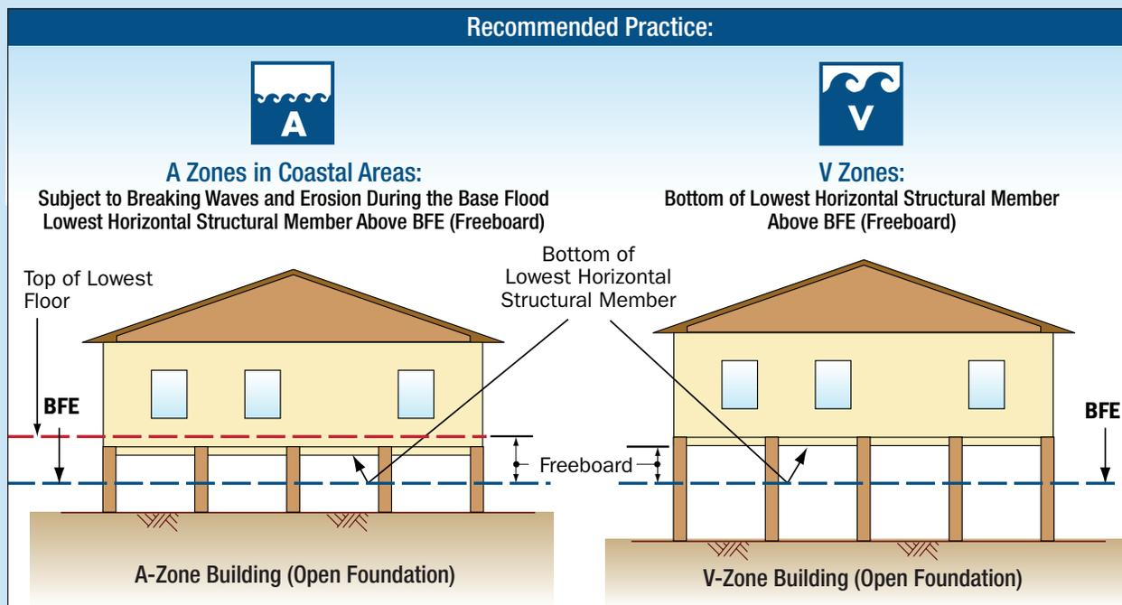
\* NFIP minimum elevation requirements: A Zones – elevate top of lowest floor to or above BFE; V Zones – elevate bottom of lowest horizontal structural member to or above BFE. In both V Zones and A Zones, many people have decided to elevate a full story to provide below-building parking, far exceeding the elevation requirement. See Fact Sheet No. 1.2 for more information about NFIP minimum requirements in A Zones and V Zones.
