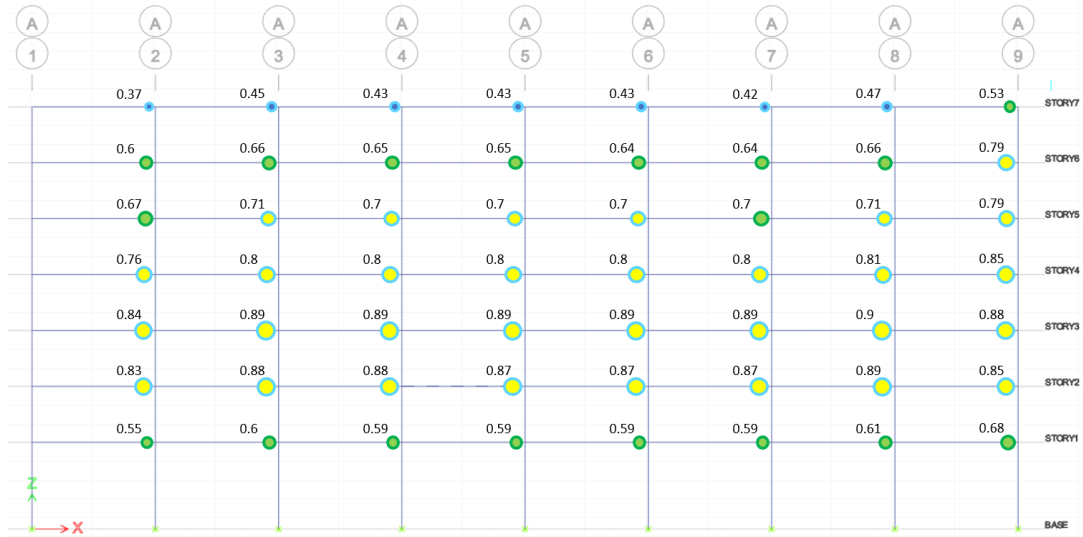
Figure 1-58 Acceptance ratios beam negative moment, ASCE/SEI 41: BSE-2N, soil takes tension (CP).
