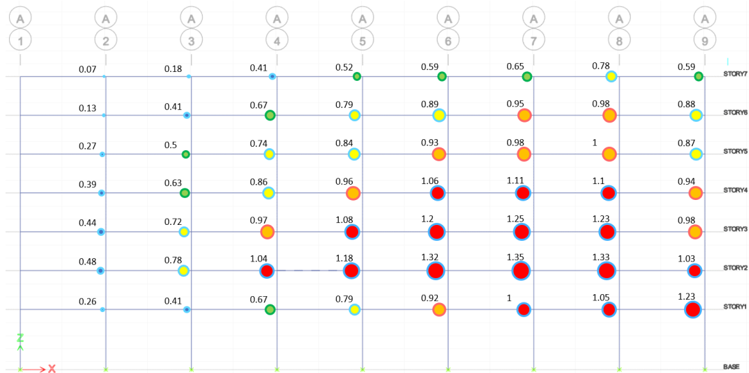
Figure 1-59 Acceptance ratios beam negative moment, ASCE/SEI 41: BSE-2N, soil compression only (CP).
