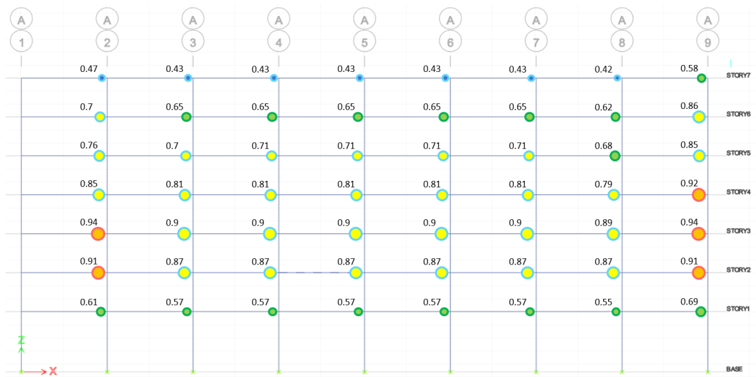
Figure 1-57 Acceptance ratios beam negative moment, ASCE/SEI 41: BSE-2N, fixed base (CP).
