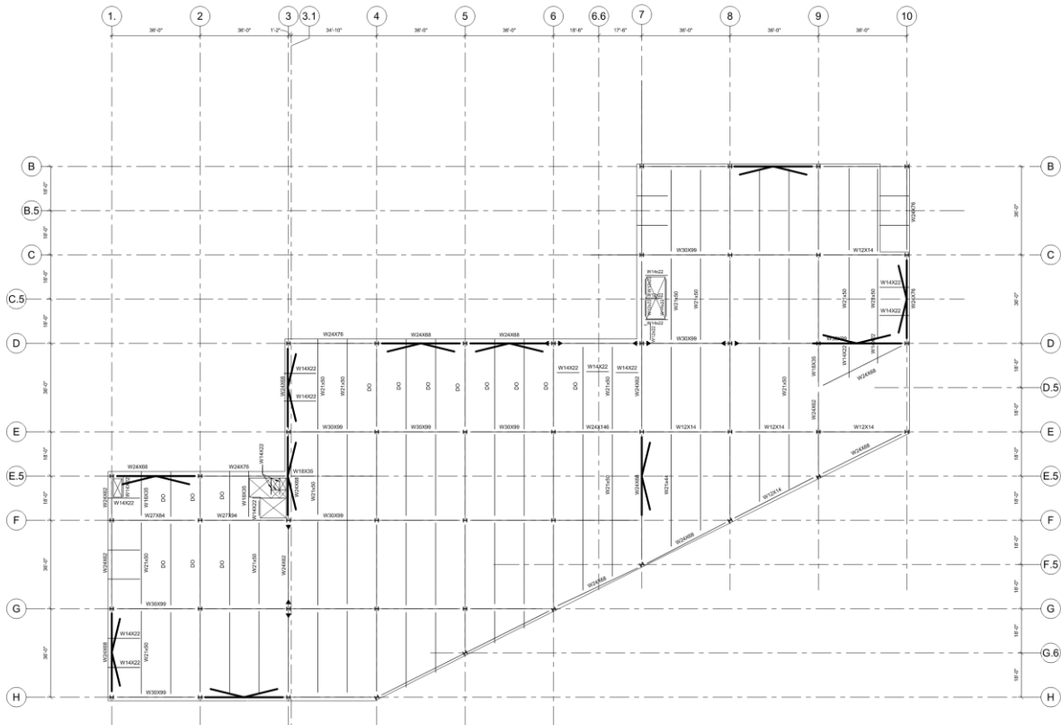
Figure 1-4 Braced frame building plan.
