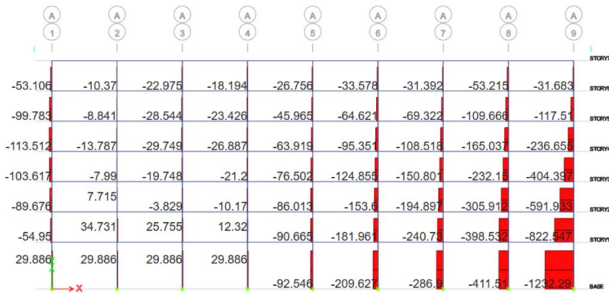
Figure 1-54 Column axial load, LC: 0.9D + E (BSE-2N), soil no tension, k_{sv} = 0.1 kci.
