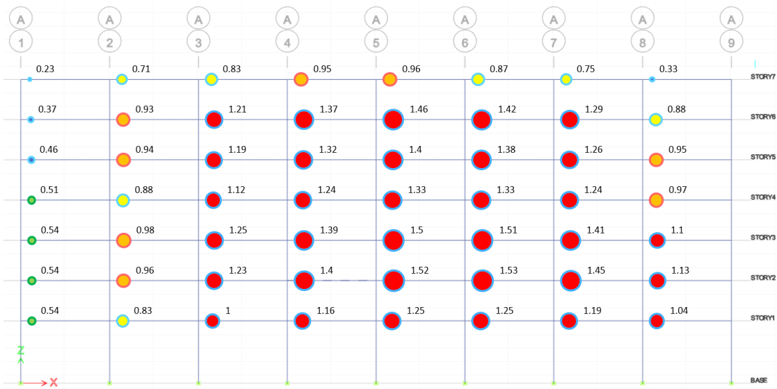
Figure 1-63 Acceptance ratios beam positive moment, ASCE/SEI 41: BSE-2N, compression only (CP).
