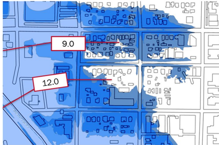
Figure 3: FFRMS Freeboard Raster Attribution. Freeboard grids of 0 to +3 feet shown in light to dark blue in grid at left, and in map at right. Cross-sections with WSELs also shown on map.
