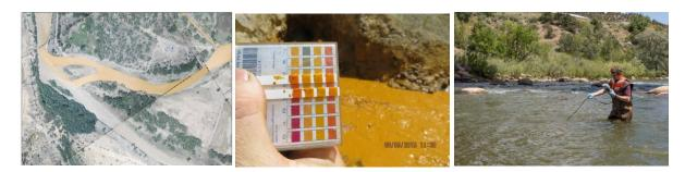
Figure 31: Chemical contamination and environmental testing of the Aminas River (Colorado) following a mining wastewater spill
