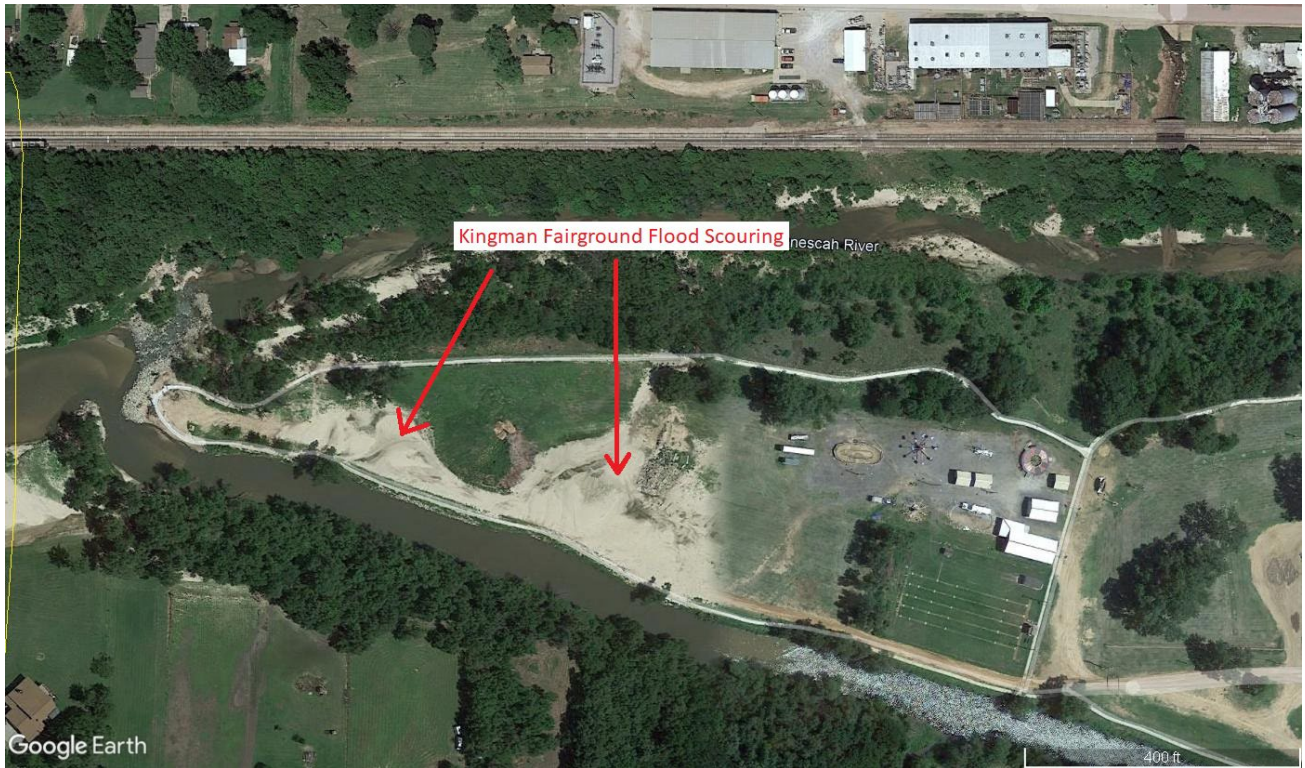
Figure 5. Aerial location view of City of Kingman Parks – Kingman Fairgrounds Park (West Side) 2019 flood scouring Source: Google Earth Pro – (Imagery date 6/27/2019)
